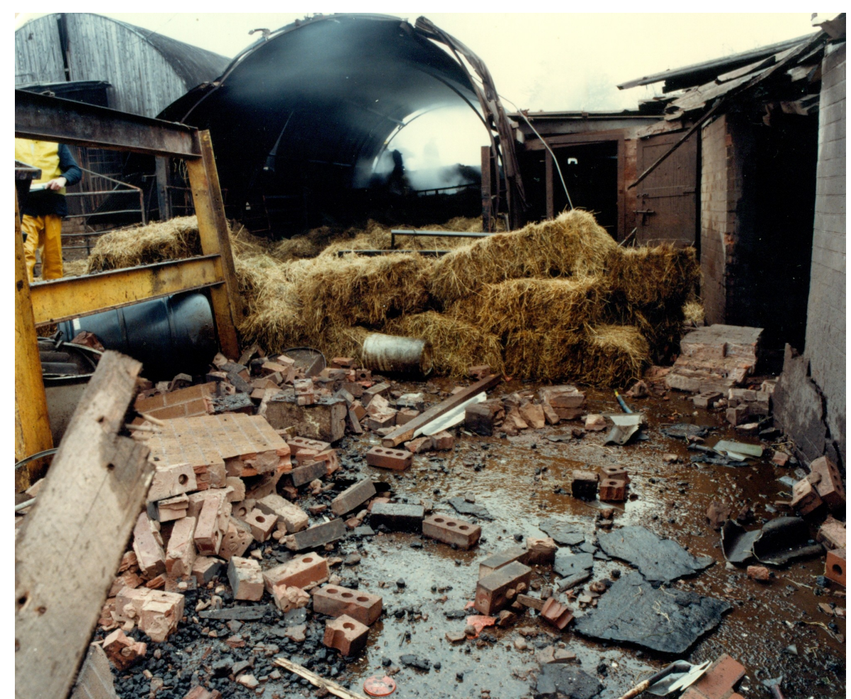
The boiler at Fields Butchers’ Lake Street abattoir had exploded, flying through the air.
